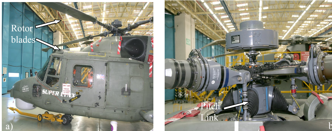
Fig. 2: a) Rotor blades of the Lynx Helicopter; b) Location of the Pitch Link
