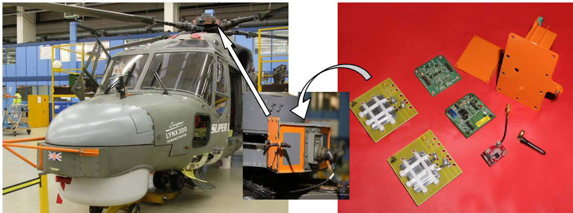
Fig. 8: WISD hardware and installation on the helicopter.
